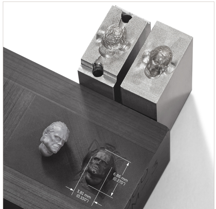
Figure 1. Electrode, cavity, and molded part with lifelike facial features
