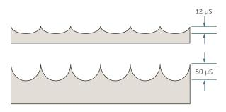
*Figure 9. The amount of on-time determines the depth of the spark craters. Longer on-time creates a deeper heat-affected layer.*
