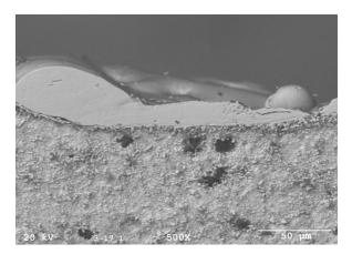
Figure 8b. 25 amps applied to the EDM cut.
